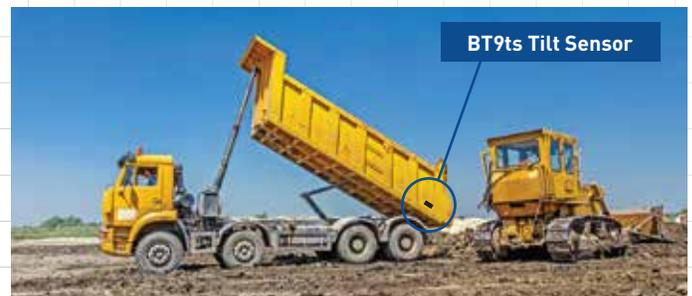
Once you have the dump body at 50% of the total dump cycle, push and release the red button. You should see the RED LED blink, indicating that the angle of the dump bed was stored in the BT9ts. If you make a mistake, just repeat the process, as any new angle value will overwrite the existing value in the BT9ts.
