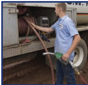
Multi-Pump tallies fuel or consumables dispensed per machine. It works in conjunction with a pulse flowmeter.
